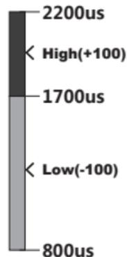
**Gyro Off Mode:** Position low, FC120 outputs receiver's signal directly
