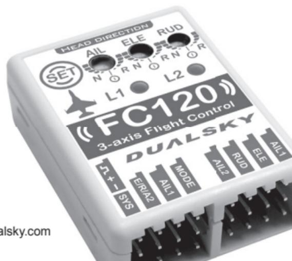
**Thank you for using Dualsky FC120 Flight Control System. This gyro is equipped with latest MEMS gyroscope, 32-bit MCU and Dualsky original algorithm. It features at mini dimensions, high sensitivity and friendly user interface, more features are listed below:**
